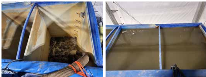
Figure 2: Photos taken while filling the sediment container with the water from Arlanda Airport. The photo to the right shows the untreated water in the sediment container.
